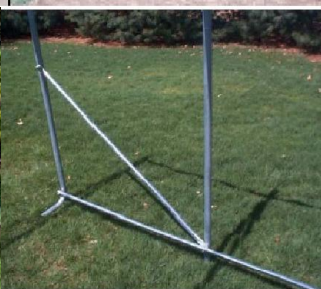
Pull U-Bolt & Anchor Loop up on Arch Base and Tighten
